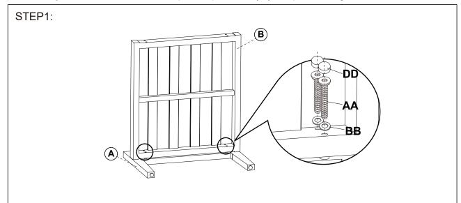
Attach the seat panel (B) to the leg (A) with bolts and washers.
