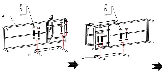
Step 2: Put the Right Leg(Part C) to the frames and assemble it with Bed(Part A) by Washers(Part E), Screws(Part D) and Screw Covers(Part F). After all hardware have been assembled, fully tighten each one with the Allen Key. After assembly, your product is ready for use.
