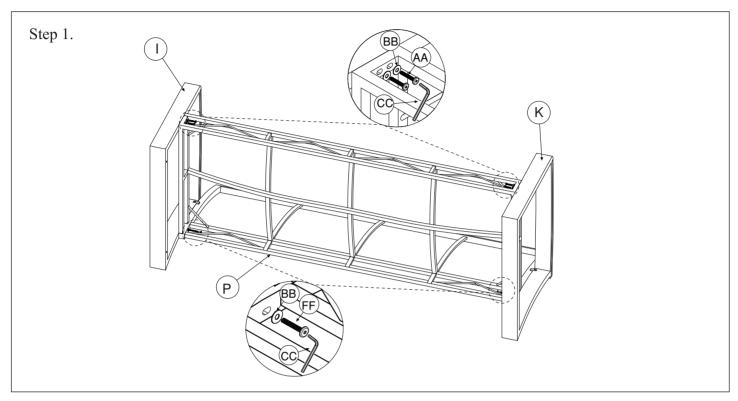
Assemble the side frame (I & K) into the seat frame (P) by bolt, flat washer. Using allen key to tighten all bolts
