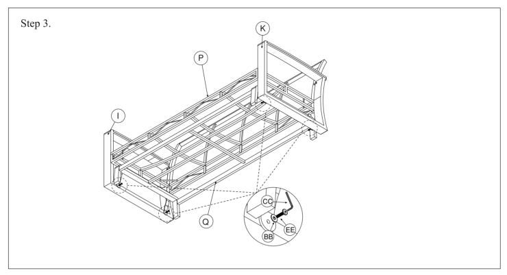
Assemble the glider (Q) into the side frame (I&K) by bolt, flat washer. Using allen key to tighten all bolts
