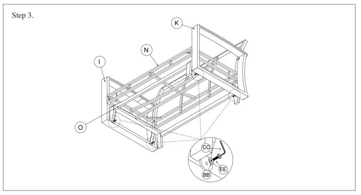
Assemble the glider (O) into the side frame (I&K) by bolt, flat washer. Using allen key to tighten all bolts
