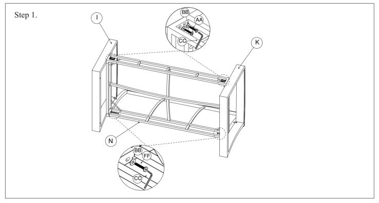
Assemble the side frame (I & K) into the seat frame (N) by bolt, flat washer. Using allen key to tighten all bolts
