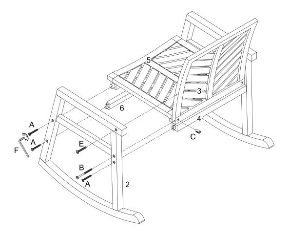
Attach part 2 to part (3, 4, 5, 6) using bolt (A, B, E) and nut (C) with hex key (F) per diagram .
