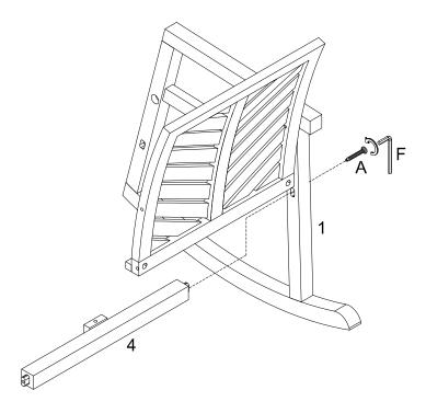
Attach part (4) to part (1) using bolt (A) with hex key (F).
