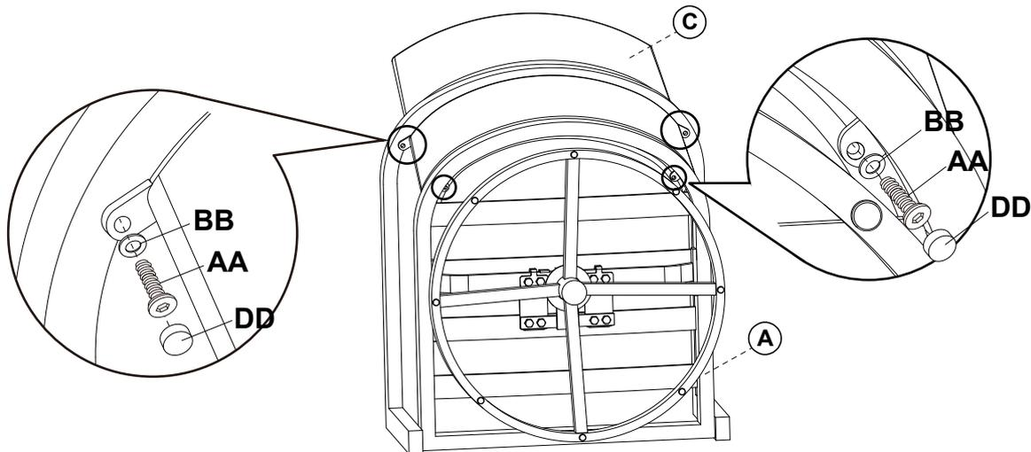
Attach the back panel (C) to the seat panel (A) with bolts and washers.
