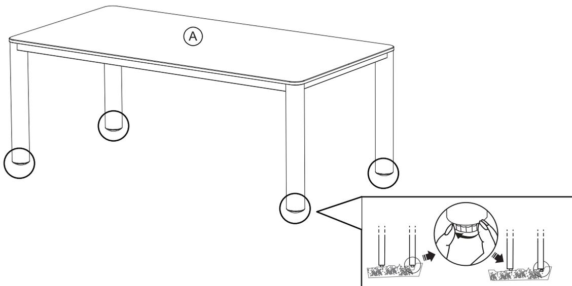
Adjust the foot leveler. Assembly complete.
