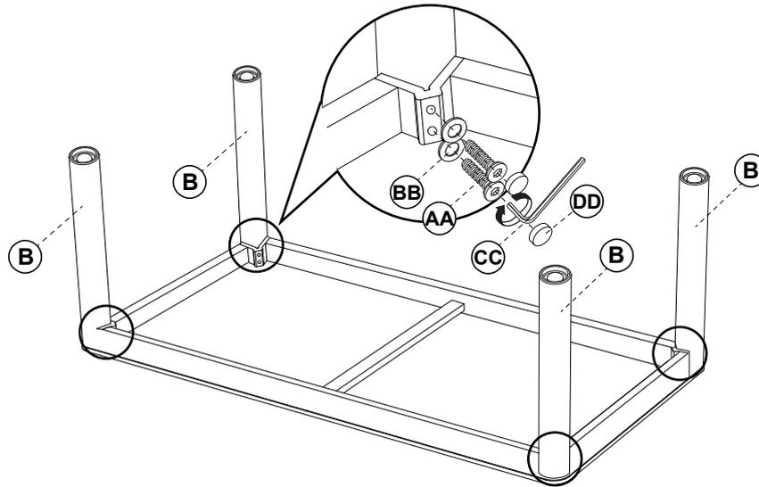
Attach the table leg (B) to the table top (A) with bolts and washers, using allen key to tighten all the bolts.
