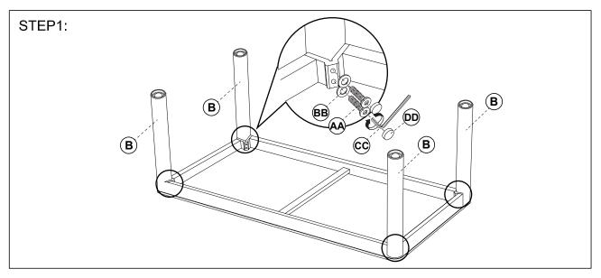
Attach the table leg (B) to the table top (A) with bolts and washers, using allen key to tighten all the bolts.
