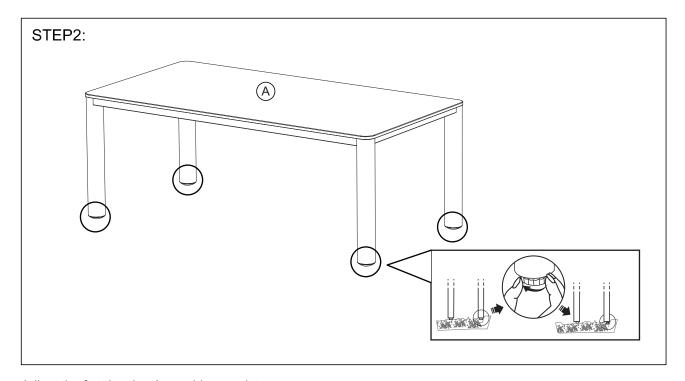
Adjust the foot leveler. Assembly complete.
