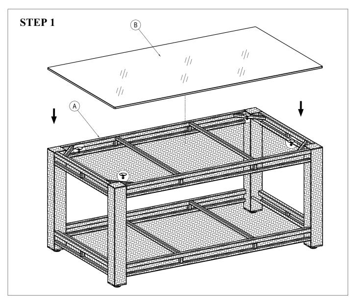
Put the glass top (B) is on the main frame (A) Assembling Completed.
