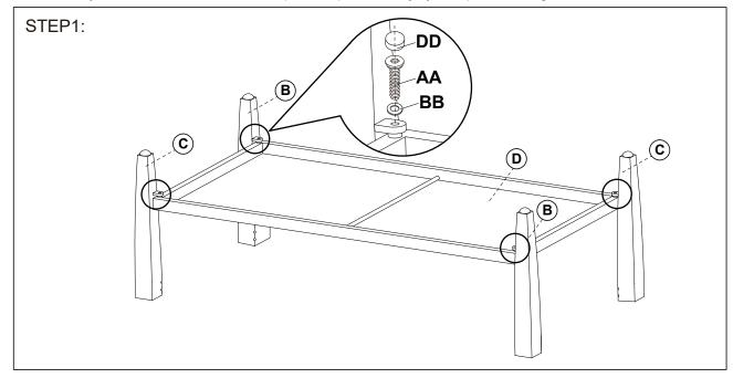
Attach the shelter(C) to the leg(B) with bolts and washers.
