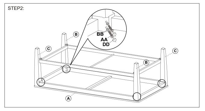
Attach the leg(B) to the top(A) with bolts and washers.
