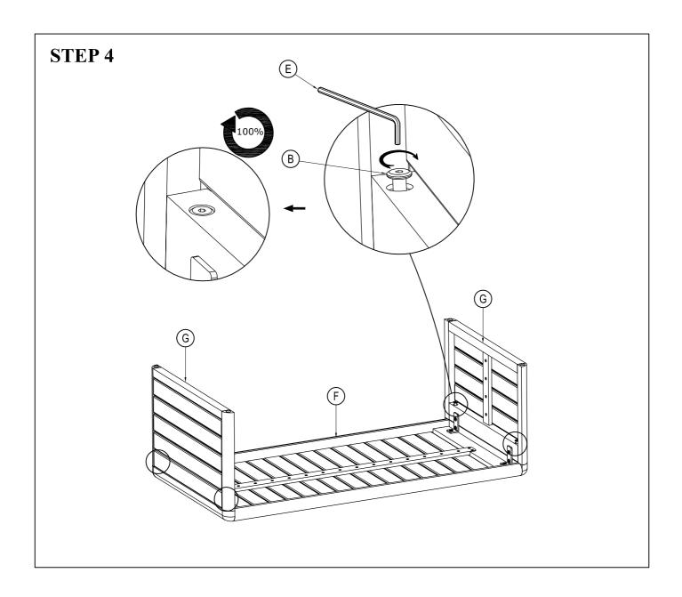
Tighten F-Bolt (B) with Allen key (E) to 100% tightness.
