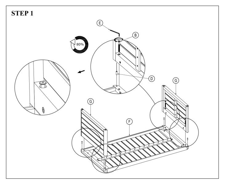
Attach table leg frame (G) to the table top frame (F) with F-Bolt (B), Wooden Dowel (D). Tighten with Allen key (E) to 80% tightness.
