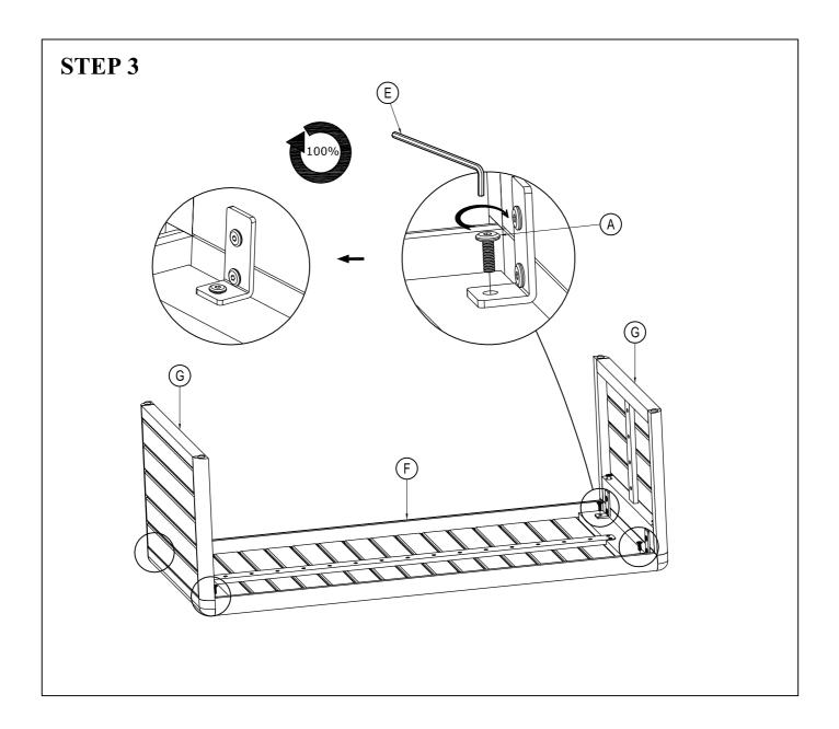
Tighten F-Bolt (A) with Allen key (E) to 100% tightness.
