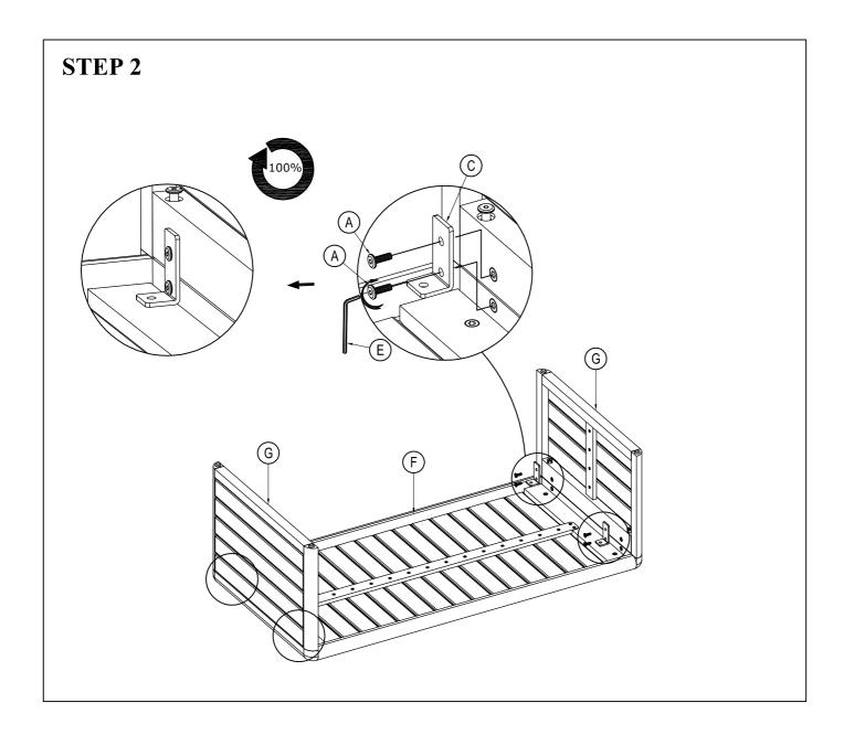
Attach Support pat (C) to the table leg frame (G) and table top frame (F) with F-Bolt (A). Tighten with Allen key (E) to 100% tightness.
