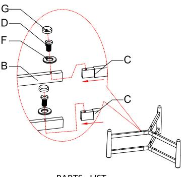
Step 2: Put the Legs(Part B) to the Table Top(Part A)together, assemble them by Washers(Part F), Screws(Part E) and Screw Covers(Part G). After all hardware have been assembled, fully tighten each one with the Allen Key. After assembly, your product is ready for use.
