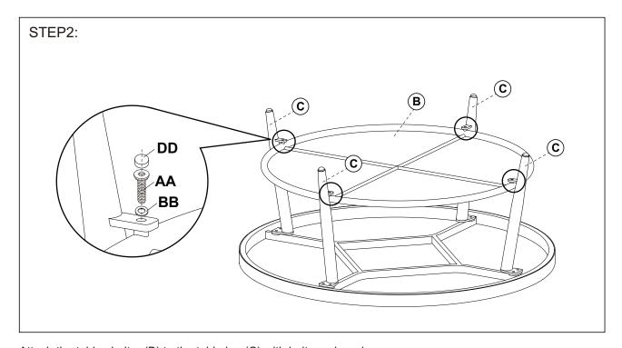
Attach the table shelter (B) to the table leg (C) with bolts and washers.
