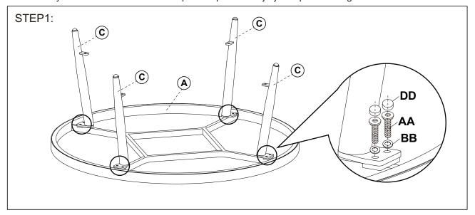
Attach the table leg (C) to the table top (A) with bolts and washers.
