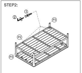
Assemble the shelf table (P2) into step 1 by bolt, spring washer, flat washer tighten bolts by allen key.
