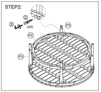
Assemble the shelf (P2) into the legs (P3) by bolt, spring washer, flat washer tighten bolts by allen key.
