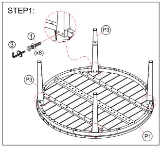
Assemple the table legs (P3) into table top (P1) by bolt, spring washer, flat washer.
