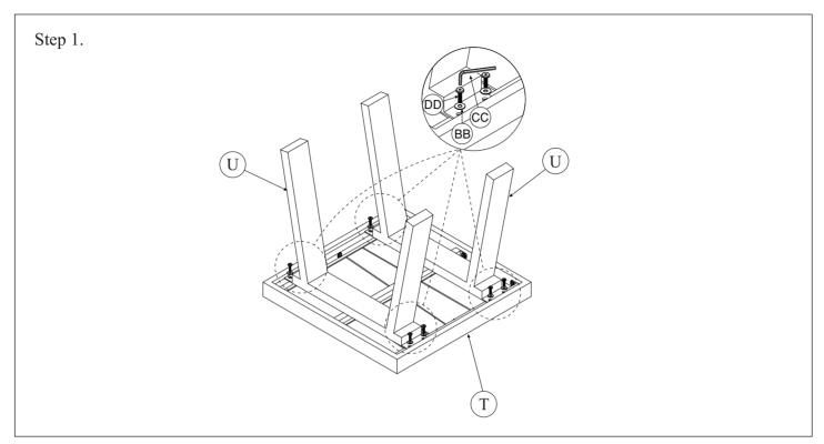
Assemble the table legs (U) into the top table (T) by bolt, flat washer. Using allen key to tighten all bolts
