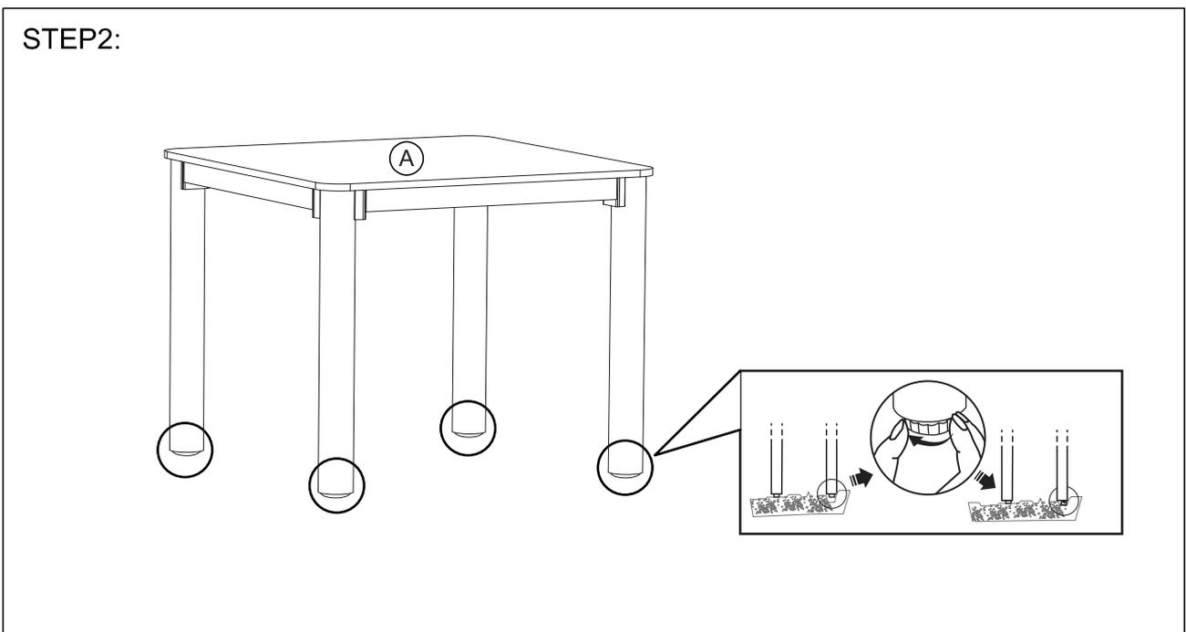
Adjust the foot leveler. Assembly complete.
