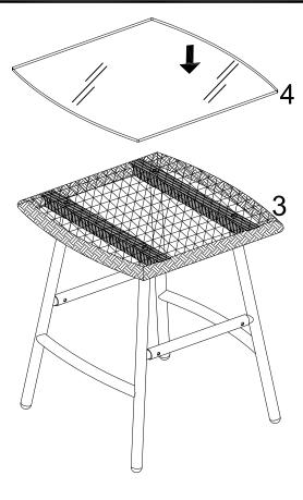
Place glass (4) carefully on top of part (3) as per diagram.
