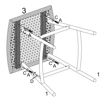
Attach part (1) to part (3) using bolt (A), washer (C) with hex key (D).
