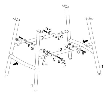
Attach part (1) to part (2) using bolt (B), washer (C) with hex key (D), and nut (E), screw cap (G) with wrench (F).
