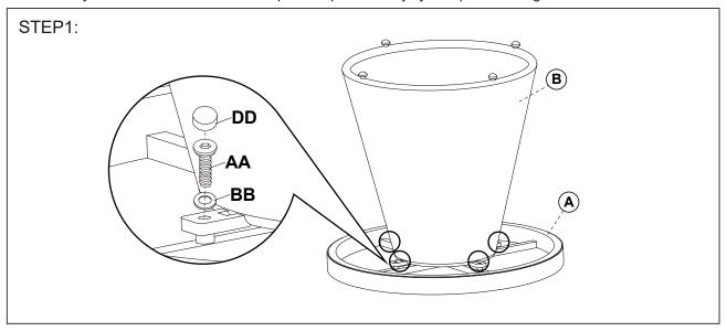
Attach the base (B) to the top (A) with bolts and washers.
