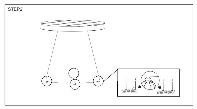
Adjust the foot leveler. Assembly complete.
