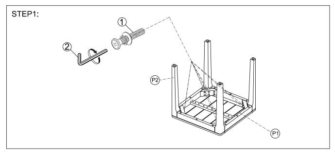
Assemple the table legs (P2) into table top (P1) by bolt, spring washer, flat washer. Tighten bolts by allen key.
