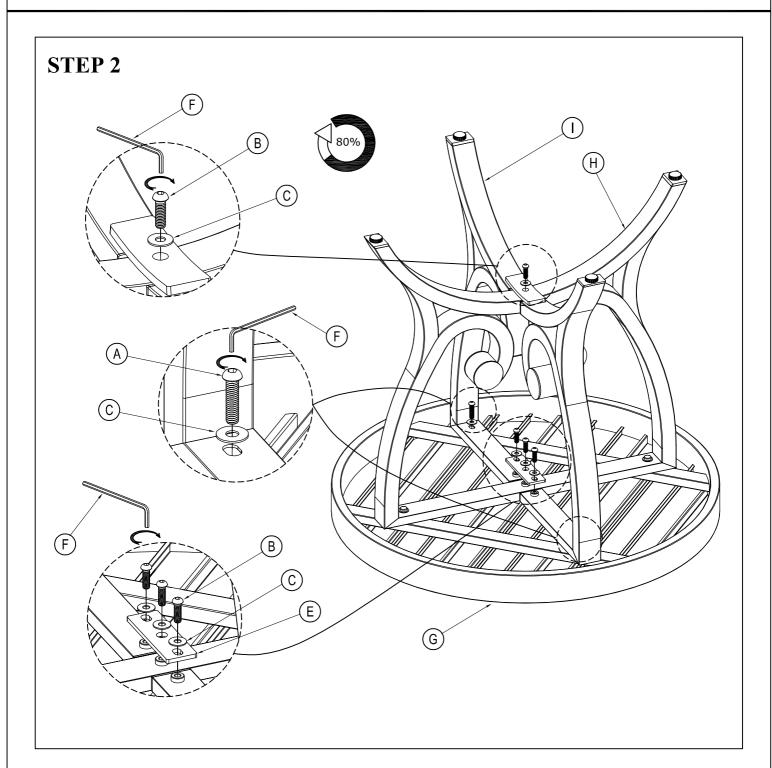
Attach the Leg Frame (I) to the Leg Frame (H) with the Mushroom-Bolt (B), Plain Washer (C) and Pat 90x30xt(4) (E). Similarly, attach the Leg Frame (I) to the Table Top Frame (G) with the Mushroom-Bolt (A), Plain Washer (C). Tighten with Allen key (F) to 80% tightness.
