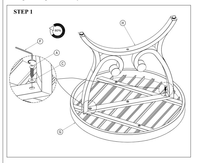
Attach the Leg Frame (H) to the below of the Table Top Frame (G) with the Mushroom-Bolt (A), Plain Washer (C). Tighten with Allen key (F) to 80% tightness
