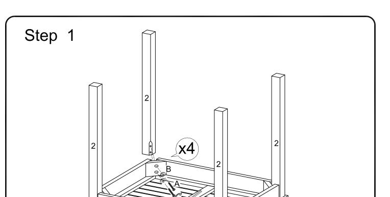
Use wrench (C) to secure top frame (1) to leg (2) with bolt (A), and washer (B).
