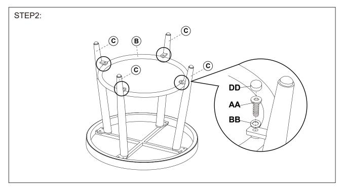
Attach the shelter (B) to the leg (C) with bolts and washers.
