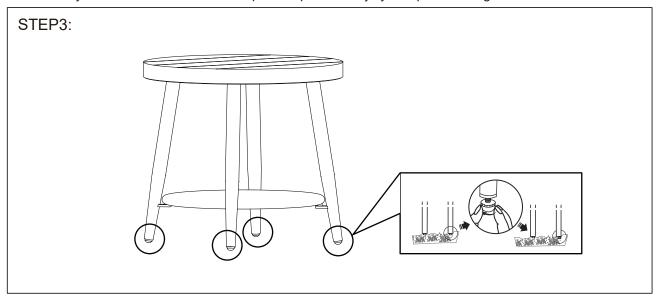
Adjust the foot leveler. Assembly complete.
