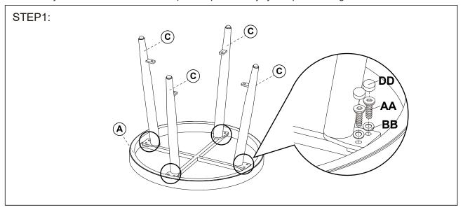
Attach the leg (C) to the top (A) with bolts and washers.
