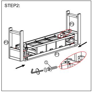
Put the bottom table facing up, assemble the leg into the table top frame.
