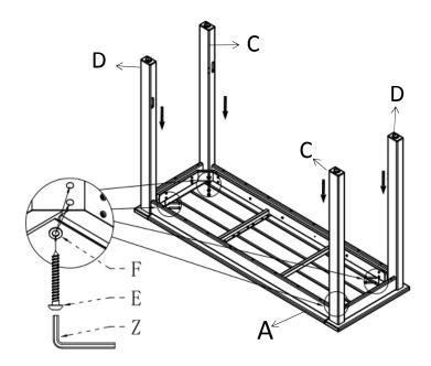
Step 2: Assemble the Top2(Part B) to the Legs(Part C&D) by Bolt(PartE) and Washer(Part F), tighten with Allen Key (Part Z).
