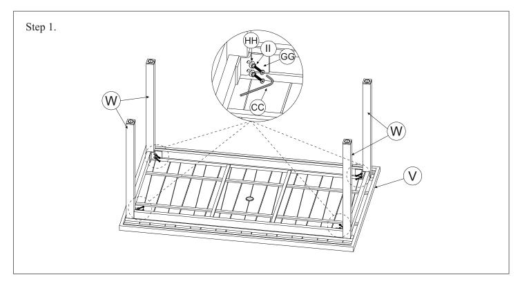
Assemble the table legs (W) into the top table (V) by bolt, spring washer, flat washer. Using allen key to tighten all bolts
