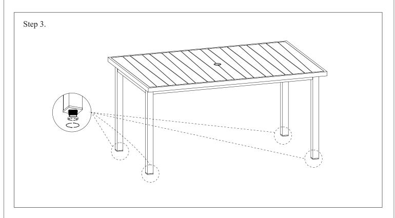
Use the adjusters at the base of the feet if the ground is uneven. Assembled complete.
