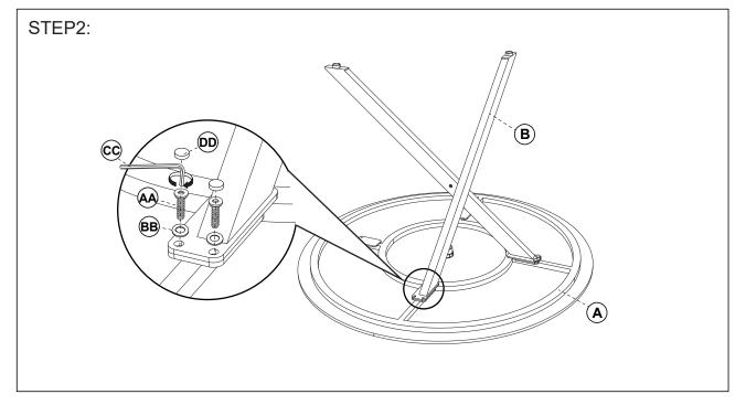
Attach the table leg (B) to the table top (A) with bolts and washers, using allen key to tighten all the bolts.
