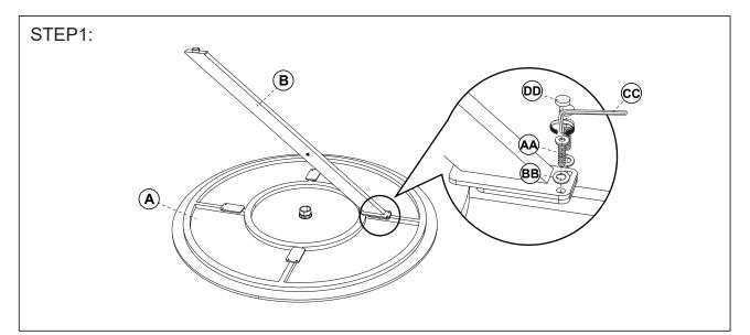
Attach the table leg (B) to the table top (A) with bolts and washers, using allen key to tighten all the bolts.
