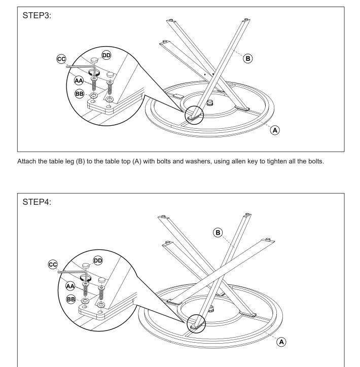
Attach the table leg (B) to the table top (A) with bolts and washers, using allen key to tighten all the bolts.
