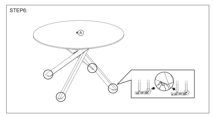
Adjust the foot leveler. Assembly complete.
