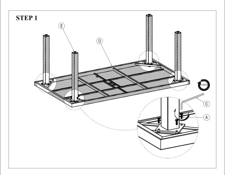
Attach the leg frame (E) to the below of the main frame (D) with the F-Bolt (A). Tighten with Allen key (C) to 100% tightness.
