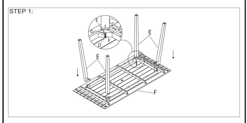
Place the Table top on the clean, soft surface as a blanket or carpet. Assemble the Leg part (A) to the Table top (B) by Flat washer, Spring washer, Hex nut (Part D,E,F) and loosely tighten with Wrench (Part G). When inserting the Hex nuts, loosely tighten each about 5-6 full turns and ensure each of the 4 Hex nuts fit well. Once all 4 are inserted and loosely tightened, proceed to fully tighten each Hex nut.
