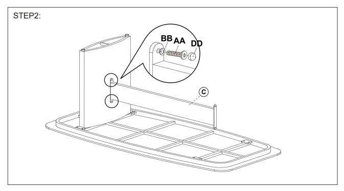
Attach the support bar (C) to the leg (A) with bolts and washers.
