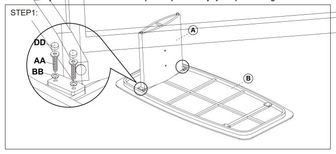
Attach the leg (A) to the table top (B) with bolts and washers.
