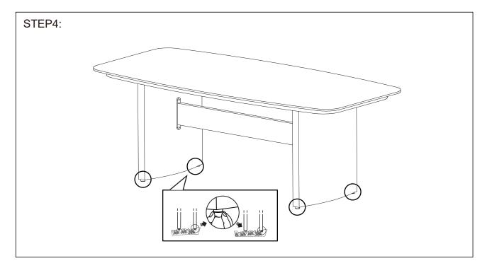
Adjust the foot leveler. Assembly complete.
