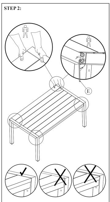
To make sure it is level, a person adjusts the chairs legs and the table top deflected, other use allen key E to tighten all bolts.
