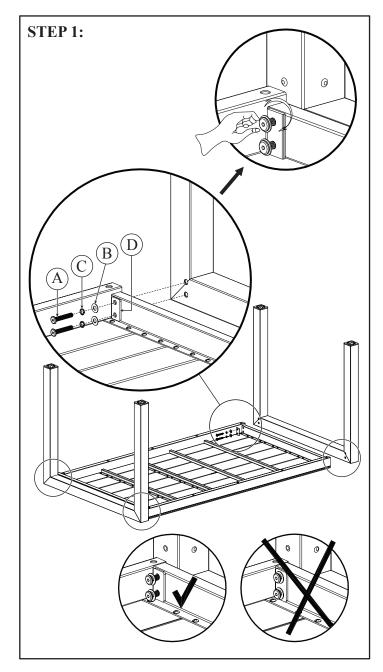
Attach the table legs to assembled the table top with F-bolt A, Spring washer C, Plain washer B and support pat D. Hand tighten only.
