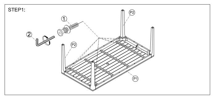
Assemple the table legs (P2) into table top (P1) by bolt, spring washer, flat washer. Using allen key to tighten all bolts.
