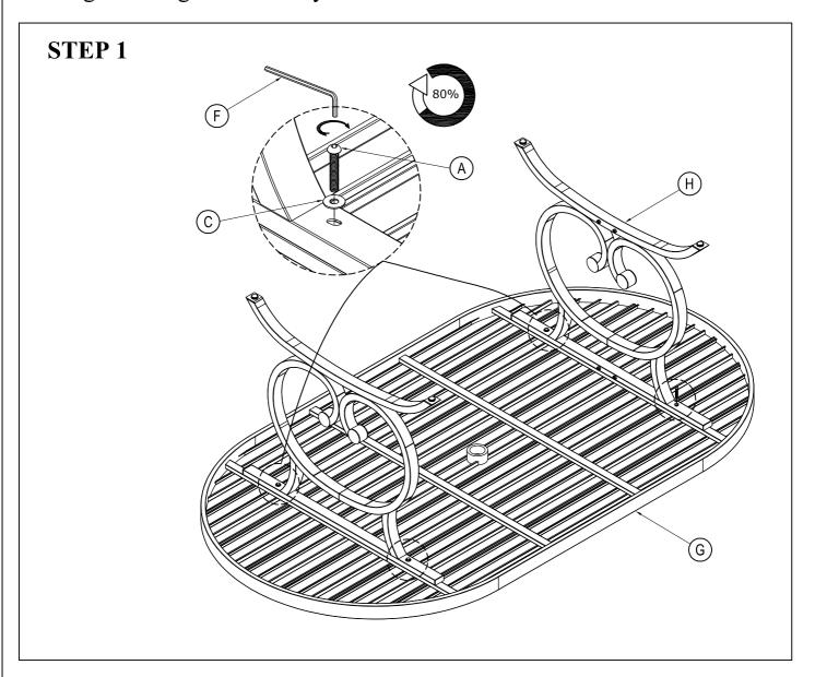
Attach the Leg Frame (H) to the below of the Table Top Frame (G) with the Mushroom-Bolt (A), Plain Washer (C).
