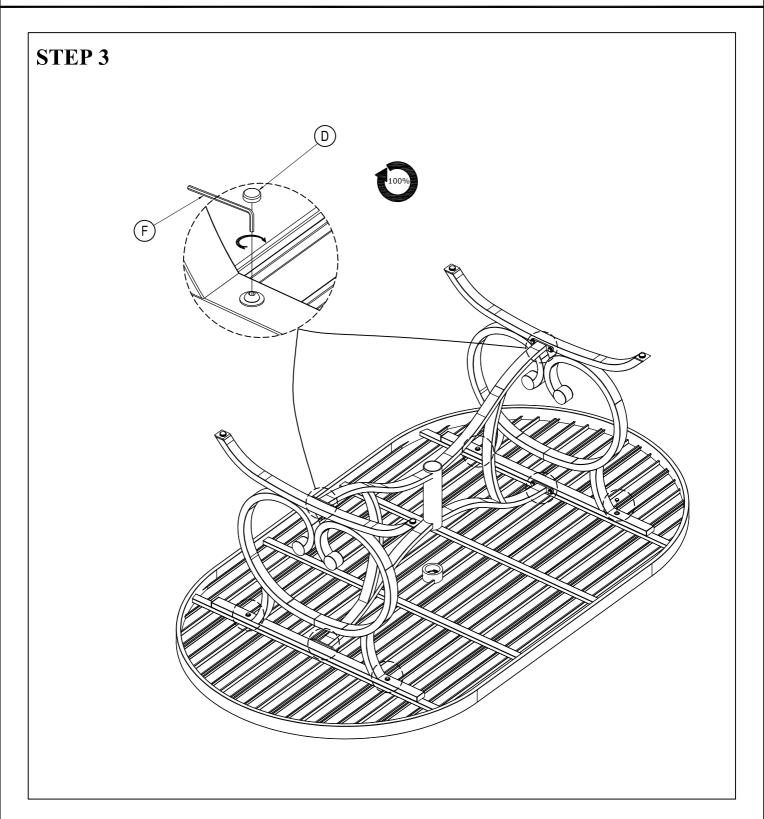
Tighten 100% tightness all positions. Attach Bolt Cap (D) on the Mushroom- Bolt.
