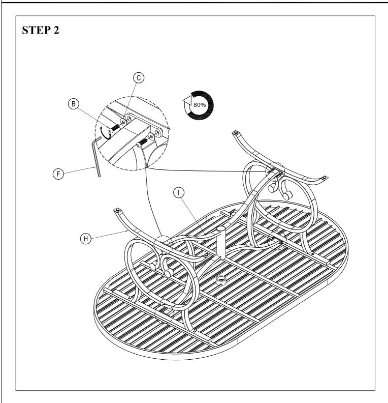
Attach the Support Leg Frame (I) to the Leg Frame (H) with the Mushroom-Bolt (B), Plain Washer (C). Tighten with Allen key (F) to 80% tightness.
