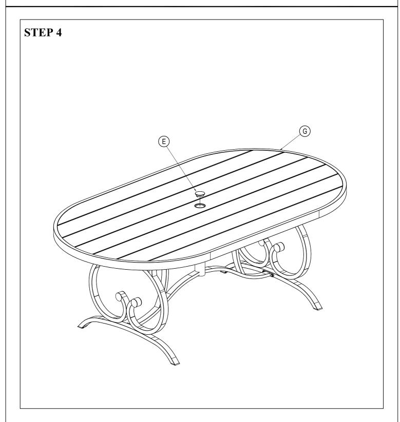
Attach the Umbrella Hole Plug (E) to the Table Top Frame (G). Assembling Completed.
