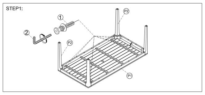
Assemple the table legs (P2) into table top (P1) by bolt, spring washer, flat washer. Using allen key to tighten all bolts.
