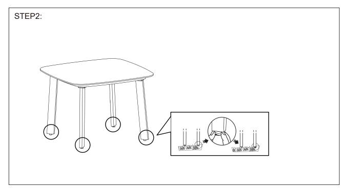
Adjust the foot leveler. Assembly complete.
