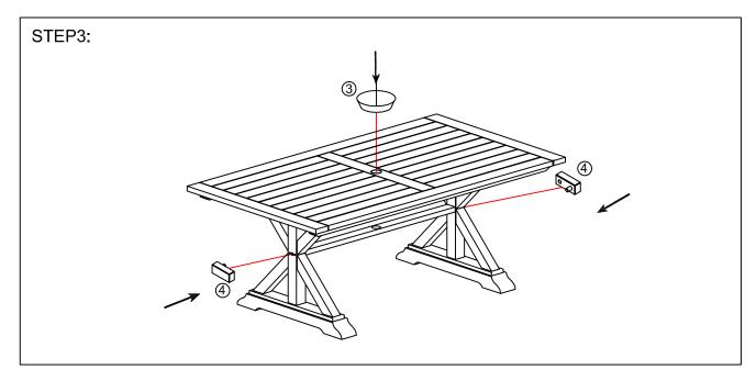
Turn the table over, put parasol cap (3) into the table top. After that put the wood plug (4) into the leg and finish.
