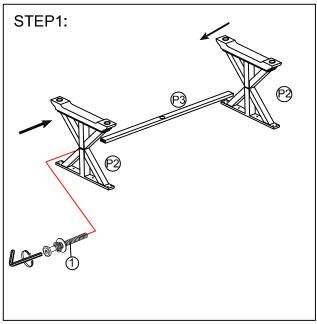
Assemble the cross bar (P3) into the leg. Note: Do not fully tighten the bolts untill the last step.
