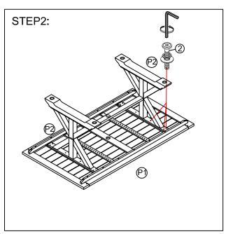
Put the bottom of table up, assemble the leg into table top. Tighten the bolts.
