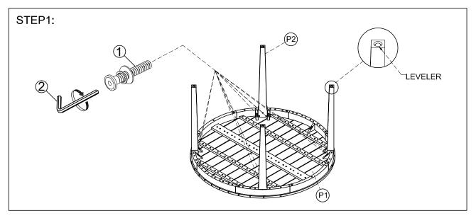
Assemble the table legs (P2) into the table top (P1) by bolts, spring washer, flat washer. Using allen key to tighten all bolts.
