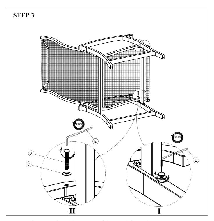
Tighten with Allen key (E) to 100% tightness (Figure I)
