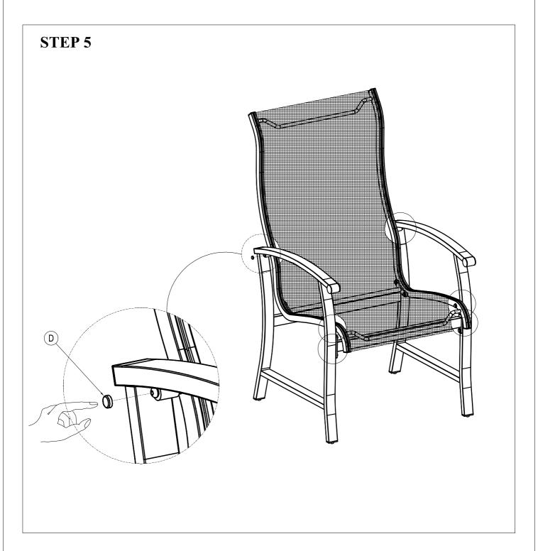
Attach Bolt Cap (D) on the Mushroom- Bolt. Assembling Completed
