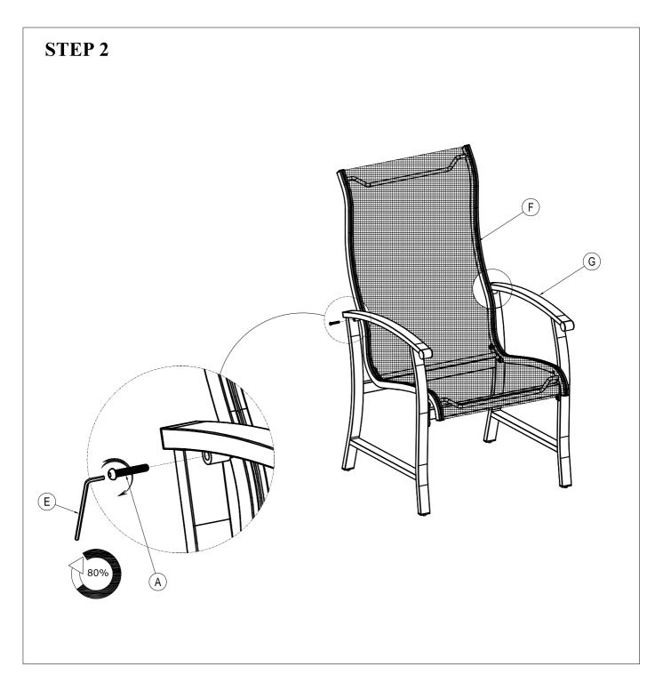
Attach the Back frame (F) to the Leg frame (G) with the Mushroom-Bolt (A). Tighten with Allen key (E) to 80% tightness.
