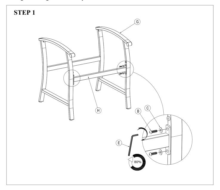
Attach the Support frame (H) to the Leg frame (G) with the Mushroom-Bolt (B), Plain Washer (C). Tighten with Allen key (E) to 80% tightness.
