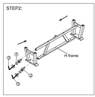
Assemble the H frame into the legs.
