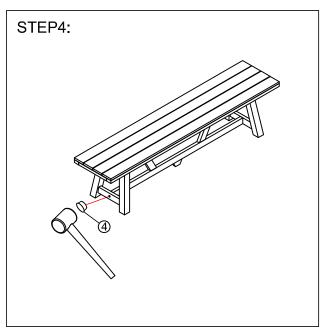
Turn the bench over and use the rubber hammer to put the wood plug into the leg and assembly completed.
