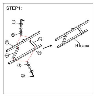
Assemble the short support bar (P4) into the support bar (P3) and the cross bar (P5).
