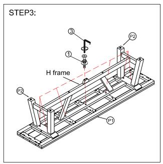
Put the seat frame bottom of Bench up, assemble the leg frame into Bench frame. And tighten all bolts.
