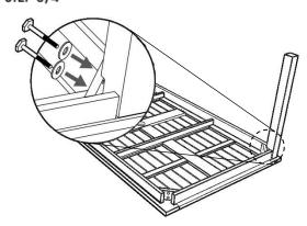
Insert the bolt through a washer from the corner-block onto the leg. Tighten it firmly with 6mm Allen Key, but be careful not to overly tighten it as the wood might crack.
