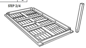
Align and insert 1 Leg section into the corner-block.
