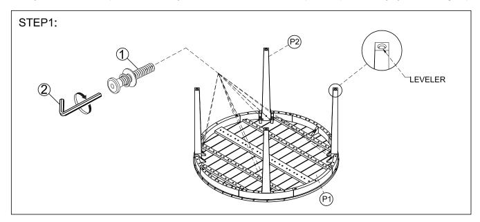
Assemble the table legs (P2) into the table top (P1) by bolts, spring washer, flat washer. Using allen key to tighten all bolts.
