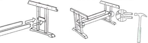
Use the hammer to tap 2 dowels into the pre-drilled holes at the ends of the rails. Total 8 dowels.
