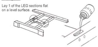
Open the small bottle with glue and apply some glue in a zig-zag pattern on THE SIDES of the 2 mortized holes.
