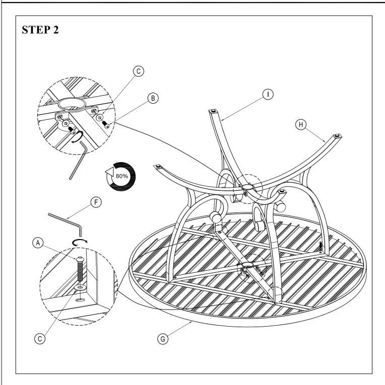
Attach the Leg Frame (I) to the Leg Frame (H) with the Mushroom-Bolt (B), Plain Washer (C). Similarly, attach the Leg Frame (I) to the Table Top Frame (G) with the Mushroom-Bolt (A), Plain Washer (C). Tighten with Allen key (F) to 80% tightness.
