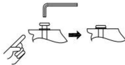
Step 1: Place the Tops(Part A & B) on a clean, soft surface as a blanket or carpet. Assemble the Legs(Part C) to the Tops(Part A & B) by Bolt(M6\*50) (Part D) and tighten with Allen key (Part Z).
