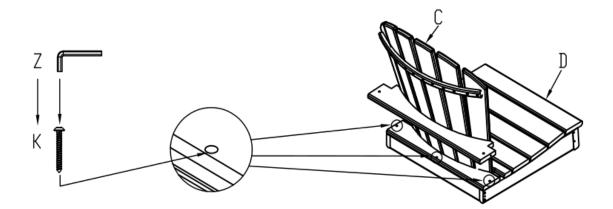
Step 2: Assemble the Right/Left Armrest with Leg(Part A&B) to the Back by Bolt(Part H&J), to the Seat by Bolt(Part G), and tighten with Allen key(Part Z).
