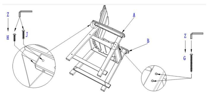
Step 3: Assemble the back leg to the Seat by Bolt(Part I), tighten with Allen key (Part Z); assemble the Front/Back footrest(Part E&F) to the legs by Bolt(Part I & H), tighten with Allen key(Part Z).
