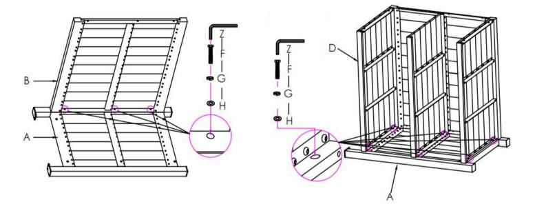
Step 2: Assemble the Right Side Panel(Part C) to the Base by Bolt(M6\*30)(Part F) and Washer (Part G&H), tighten with Allen Key (Part Z).
