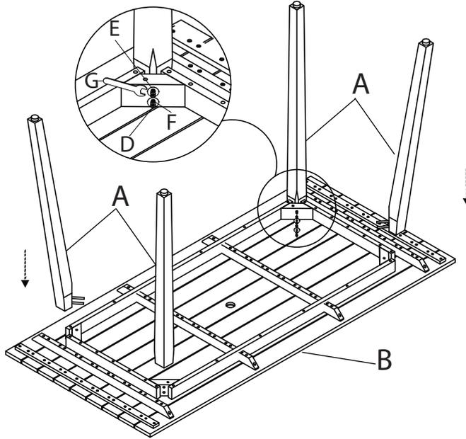
Place the Table top on the clean, soft surface as a blanket or carpet. Assemble the Leg part (A) to the Table top (B) by Flat washer, Spring washer, Hex nut (D,E,F) and loosely tighten with Wrench (G).When inserting the Hex nuts, loosely tighten each about 5-6 full turns and ensure each of the 4 Hex nuts fit well. Once all 4 are inserted and loosely tightened, proceed to fully tighten each Hex nut.
