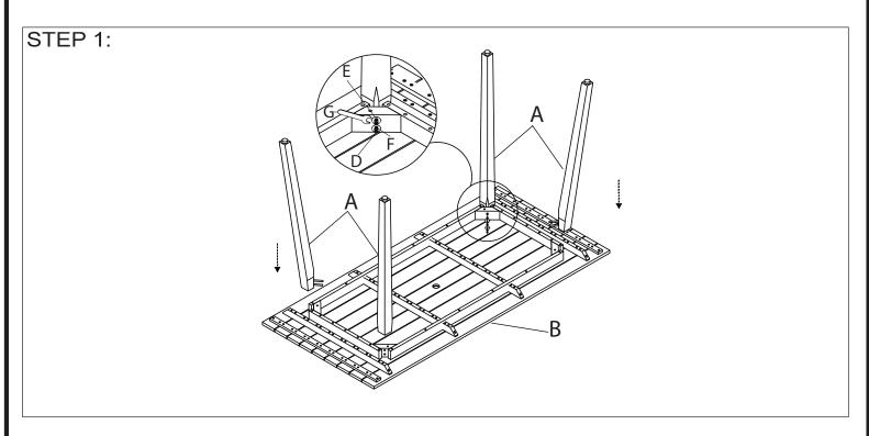
Place the Table top on the clean, soft surface as a blanket or carpet. Assemble the Leg part (A) to the Table top (B) by Flat washer, Spring washer, Hex nut (D,E,F) and loosely tighten with Wrench (G). When inserting the Hex nuts, loosely tighten each about 5-6 full turns and ensure each of the 4 Hex nuts fit well. Once all 4 are inserted and loosely tightened, proceed to fully tighten each Hex nut.
