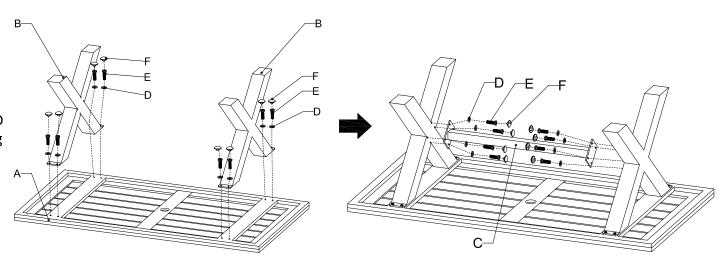
Step 2: Assemble the Support Bar (Part C) between Cross Leg by Washer & Screw (Part D and E) and loosely tightening with the Allen Key.
