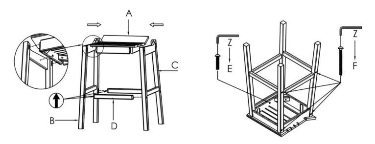
Step 2: Assemble the Right Leg(Part B) to the Seat and Foot Bar by Bolt(M6\*65)(Part F), put the Bolt(M6\*30)(Part E) into the hole on the side of Seat(Part A), and tighten with Allen Key(Part Z).
